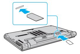
Do not touch the printed circuit on the SIM card. Be sure to hold your computer firmly before inserting or removing the card. Do not damage the SIM card in any way, either by bending or exerting pressure on the card.
